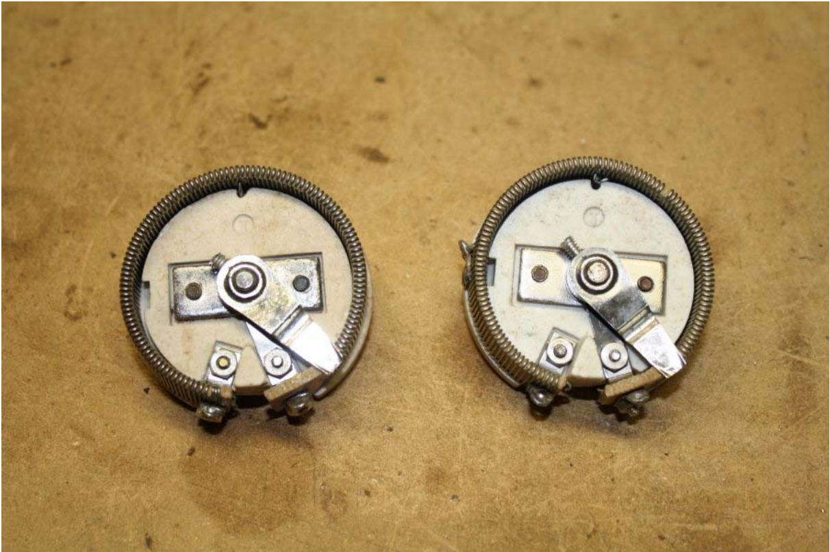
The amplifier rheostat had two breaks in the winding. Now fixed.
