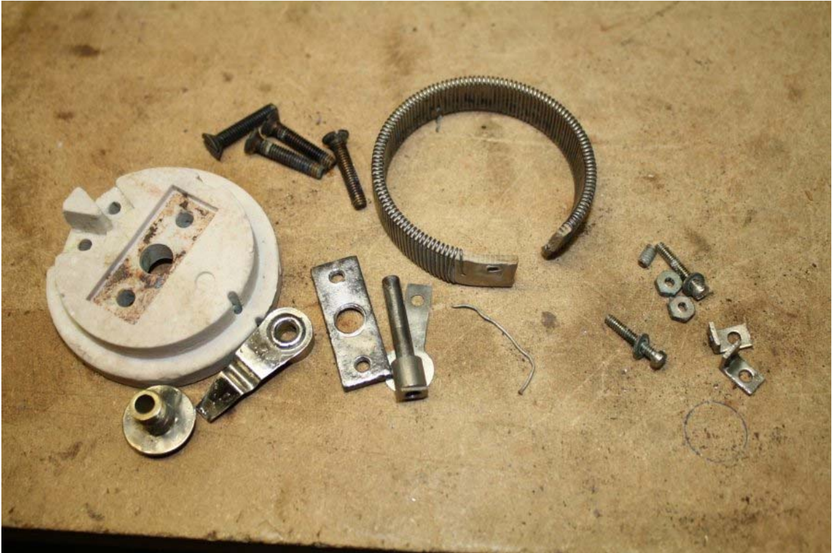
The amplifier rheostat had two breaks in the winding. Now fixed.
